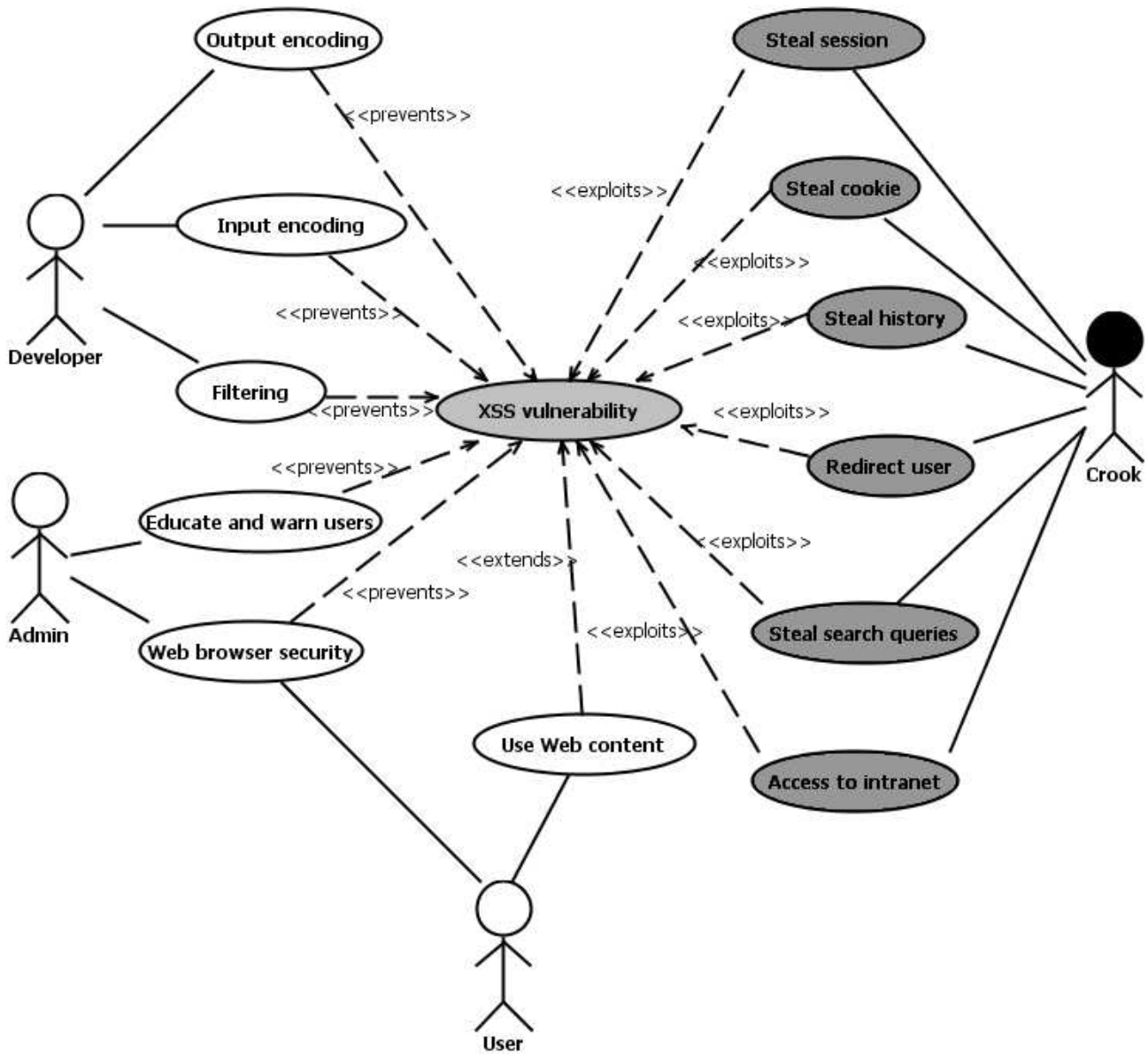
Figure 4. A use case model extended with misuse case notation to represent the threats and countermeasures of a XSS vulnerability.
